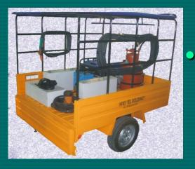
THE TRANSPORTABLE UNIVERSAL WELDING REPAIR SHOP
